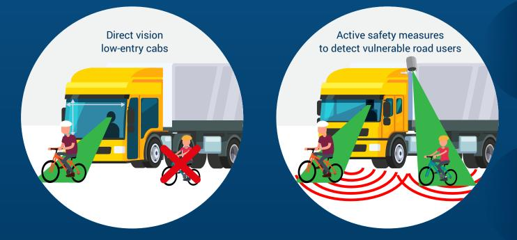
Moreover, contrary to 'direct vision' low-entry cabs, **active safety measures will actively draw the attention of the driver to the critical area or the VRUs concerned**. Even with the widest possible field of view in a low-entry cabin, a truck driver can only look in one direction at a time and still might fail to notice a pedestrian or cyclist on the other side of the vehicle.
